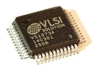
From a hardware point of view VS1073 is a pin-compatible replacement for VLSI
